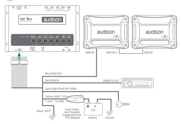
**Remark:** the **bit Ten** is internally protected by a fuse-resistor soldered on its printed circuit board. To replace it contact a service centre. Using an external fuse is recommended, though it is not required.
