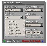
The crossover filter response corresponding to the selected channel is displayed on the graph by a red curve, as in the examples below.
