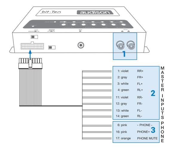
AUX IN L - R; auxiliary low-level stereo input.
