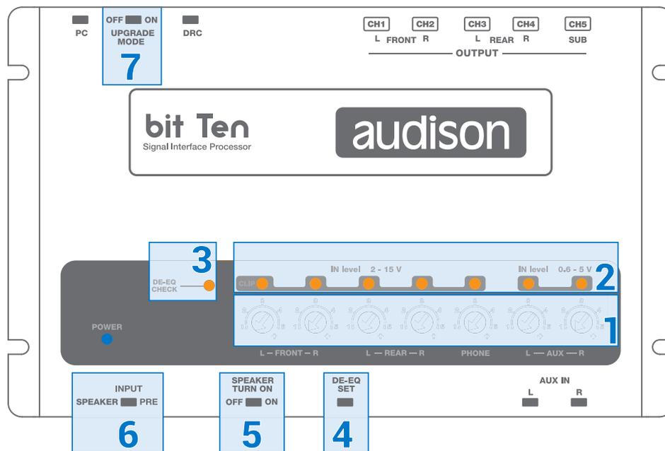
**1. IN level:** IN level: Input signals adjustments.
