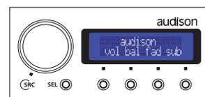
**Warning:** do not use aggressive cleaning agents or abrasive cloth to clean the display. Simply use a soft cotton cloth lightly damped with water.
