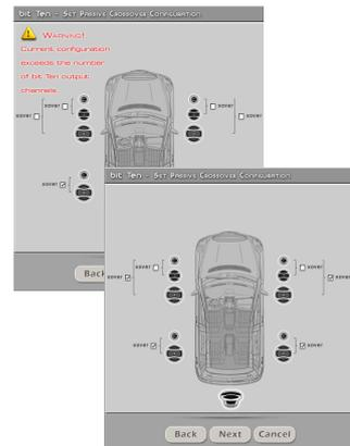
**12. Processor outputs (Ch1÷Ch5) allocation.**
