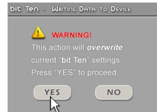
**WARNING:** before disconnecting the **bit Ten** from the PC or each time that you exit the PC Software after modifying the system configuration, always run the **Finalize to bit Ten** procedure. If you do not follow these instructions, all data entered will be lost and the device will use the previous settings.
