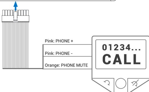
**PHONE +/-** Input compatible with the hands-free kit speaker output (see 4.2.3). Sensitivity adjustable from 2 to 15 V RMS.
