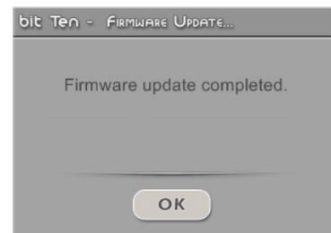
10. Start the **bit Ten** again and launch the PC software in **TARGET** mode. If the **bit Ten** firmware update has completed correctly, the dialog box will show the following indications:
