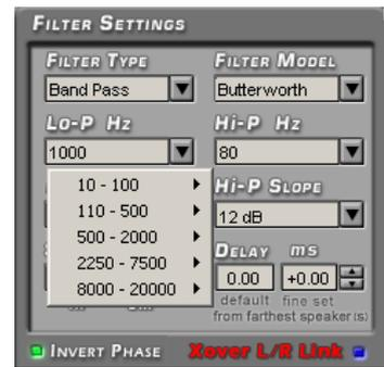
**In STANDARD mode** the crossing frequency for speakers of the same front is bound with a -3 dB crossover.
