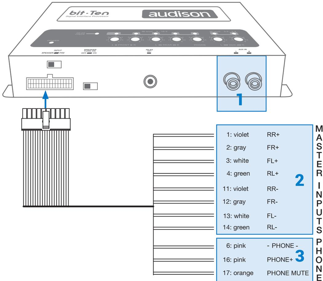
1. **AUX IN L - R;** auxiliary low-level stereo input.
