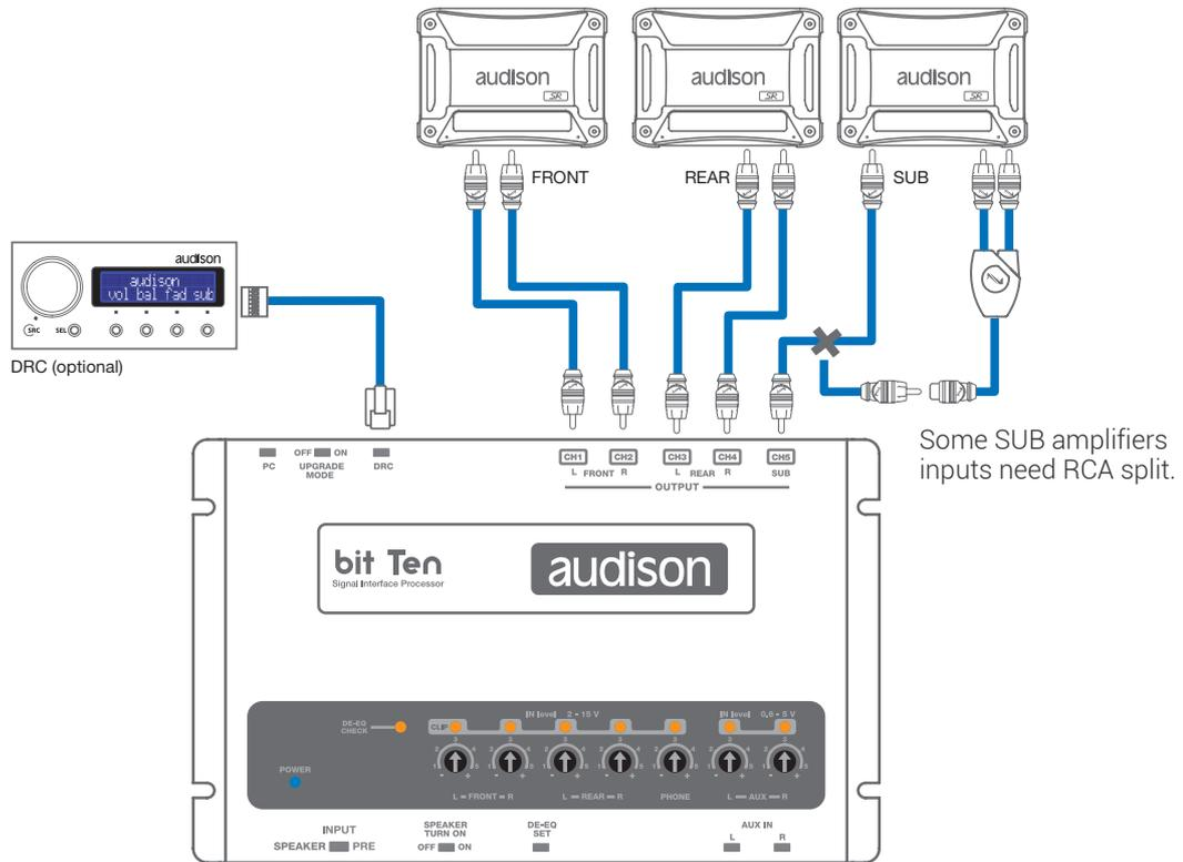
Example of a 2-way active Front + Sub amplifier's system ([see 8.2](#)).
