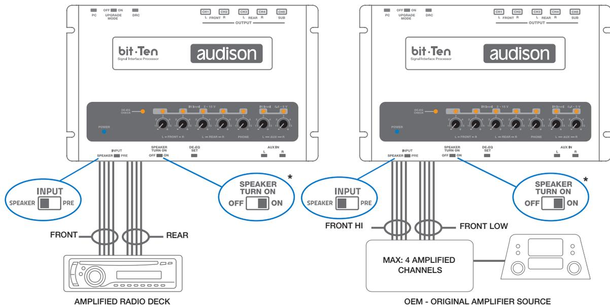
\* To disable the Speaker Turn on function on the Front Left channel, move the indicated switch to the left to "OFF" position.
