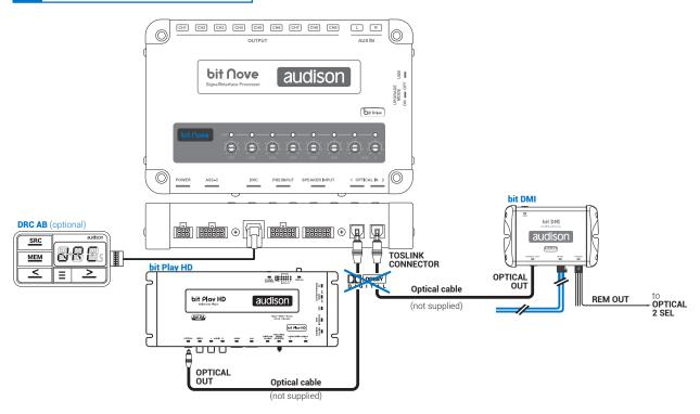
**WARNING:** the digital input accepts up to 192 kHz / 24 bit stereo PCM signals. So DOLBY DIGITAL (AC3) multi-channel signals coming from audio/video sources (such as the audio of a film in DVD) or DTS can not be reproduced. The output of these devices will therefore have to be set in STEREO mode for the signal to be reproduced.
