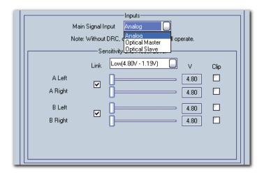
The note warns that if the DRC is not connected to the system, even selecting a digital input, when ACNet software will be switched off, only the Analog Input will operate.
