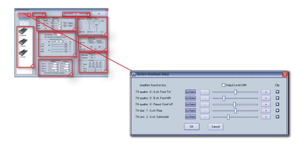
Once each single amplifier in the system has been set, it is possible to use the setup window above, which allows the sensitivity adjustment of all amplifiers of the entire system.
