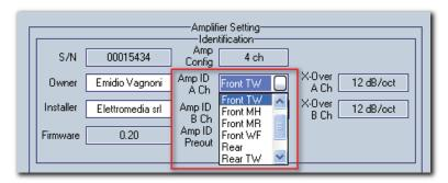
The drop-down menu displays the available values to be assigned to the amplifier depending on its configuration / functioning modes.
