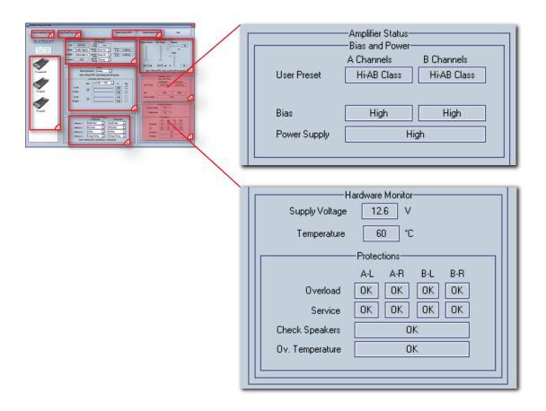
The ACNet software performs a real-time check-up of the amplifiers operating conditions.
