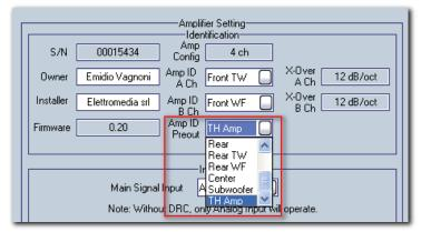
If the system is also composed by non-TH amplifiers, they can be managed by attributing an ID to the Pre Out connected to them. The menu default option is "TH AMP", because generally a TH amp (provided with its specific Amp ID already) is connected to the Pre Out.
