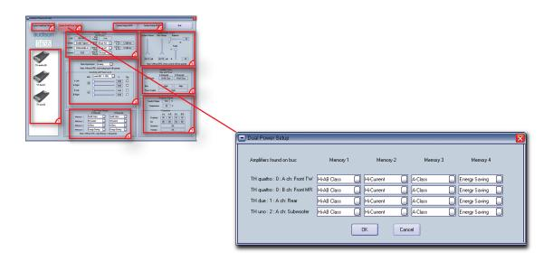
This setup enables the complete management of the operating mode of the amplifiers in the systems. The chart above presents in one window all the amplifier names and channels being used.
