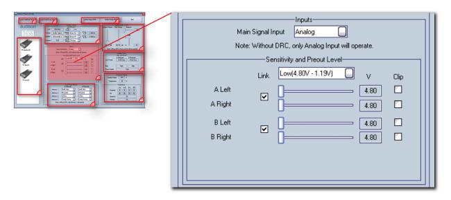
As for the ASC Setup Amplifier, it is necessary to set the system whenever wanting to use the digital input. In this area it is necessary to select the Main Signal Input for each amplifier connected to the system Example:
