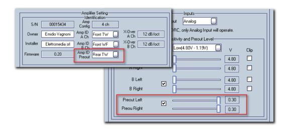
When using a non-TH amplifier to be controlled by DRC, an ID must be assigned to the Pre Out where it is connected. In this way it is still possible to manage the TH Preout sensitivity.
