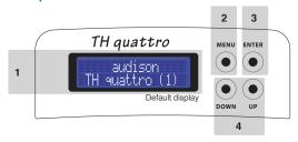
1 • TH quattro STATUS DISPLAY: it is the visual element of the ASC system, a back-lit two line 32 character LCD display; While working, it can relate all of the configuration parameters memorised by the amplifier during the installation, as well as the operational status of the amplifier.
