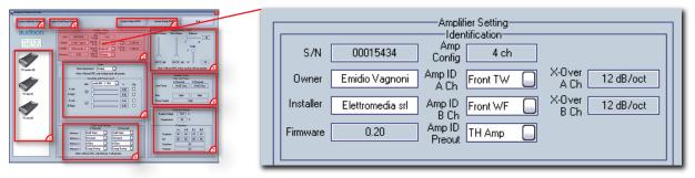
The amplifier identification provides its S/N - serial number (fixed), the owner name (free-text), the installer name (free-text) and the Firmware release included in the microprocessor inside the TH amplifier.
