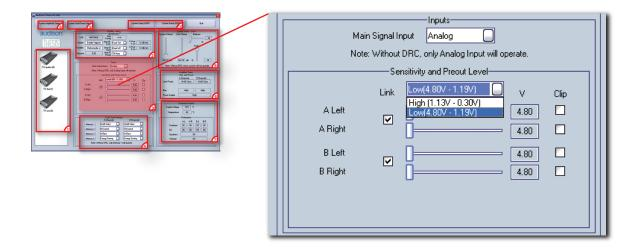
From this section featuring drop down menus, it is possible to regulate each amplifier's input sensitivity, acting also on the High/Low Level.
