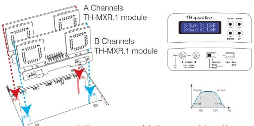
In this case you can verify both presence and slope of the crossover by checking the ASC Status Monitor, however it is not possible to modify its slope. See page 53.
