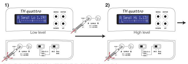
TURN THE KNOB TO REGULATE THE LEVEL OF THE A CHANNELS. PRESS THE KNOB FOR 3" TO CHANGE THE RANGE FROM HI TO LO AND VICE VERSA. IF YOU ARE USING THE IN B CHANNELS INPUT, REPEAT THE TUNING STEP ON THE B LEVELS KNOB.
